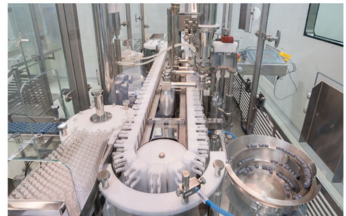
Combi fill-finish for vials, cartridges & pre-filled syringes at GMP manufacturing plant at Puducherry.
