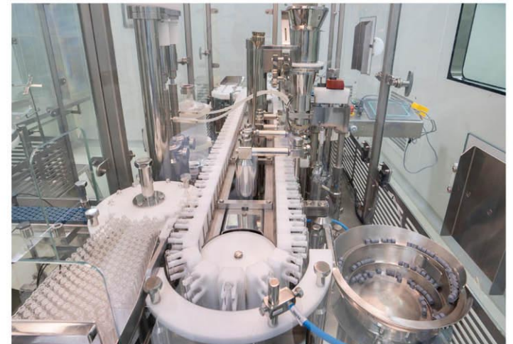
Combi fill-finish for vials, cartridges & pre-filled syringes at GMP manufacturing plant at Puducherry.
